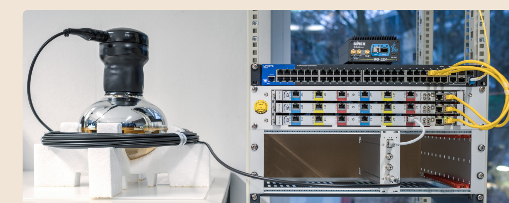
Full electronics chain with passive-base PMT, custom phantom HV supply and 250 MS s -1 ADC with GbE readout.
