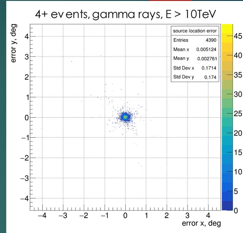
The arrival direction of particles was determined as the weighted (by image size and  $\sin\theta$  between intersection lines) average position of the points of intersection of the major axes of all ellipses.
