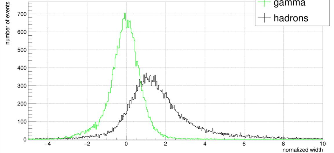
$$w = \frac{1}{N_{trig}} \times \left[ \sum_i^{N_{trig}} \frac{width_i - w_m(r_i, size_i)}{w_{90}(r_i, size_i)} \right]$$
