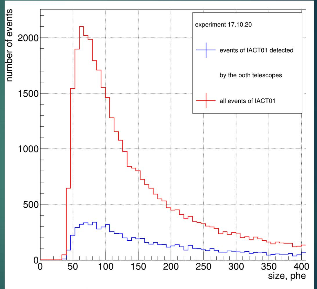
experimental and MC distribution of size of events detected by the both telescopes of the TAIGA-IACT
