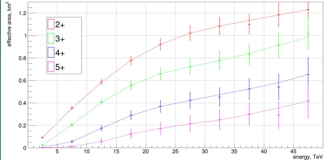
At an energy of 22 TeV in stereo mode, the effective installation area is  $\sim 0.9 \text{ km}^2$
