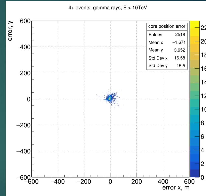
To determine the core position, the procedure for minimizing the distances to the axes connecting the image CoG and the shower arrival direction (so called *dist*) was used. In the case of triggering 4+ telescopes, the distribution RMS is  $\sim 16$  m.
