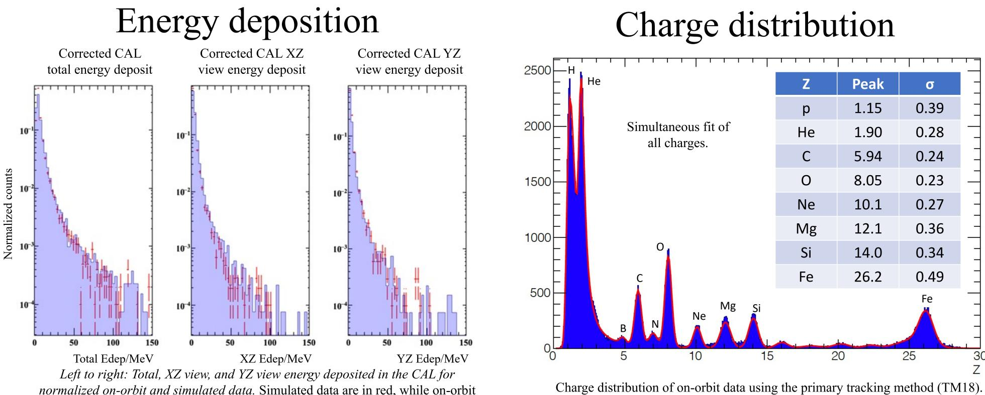
normalized on-orbit and simulated data. Simulated data are in red, while on-orbit data are in blue. The same normalization constant is used for all three distributions for on-orbit or simulated data. Event selection used the primary tracking method (TM18), required a charge identified, and total energy above 1500 MeV. Note: these CAL energy data are scaled by a factor of 6.
