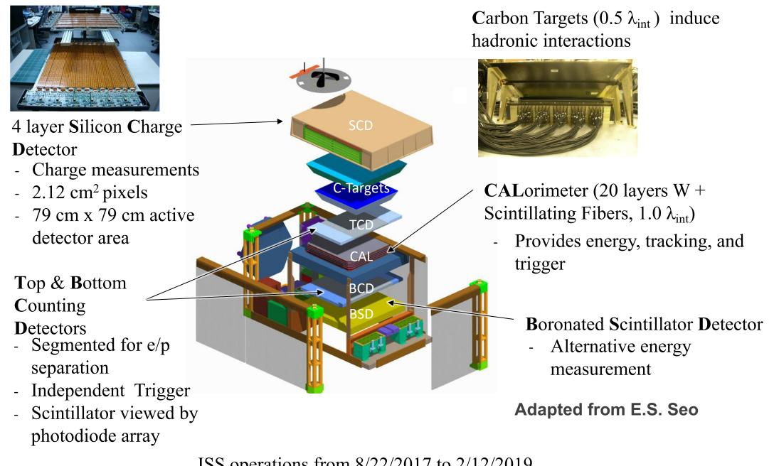
ISS operations from 8/22/2017 to 2/12/2019 CAL provides XZ/YZ tracking with 50 fiber bundles/layer.
