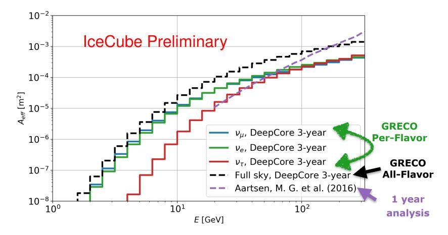
• Effective area is significantly larger than previous one-year muon neutrino charged-current selection used for low energy transients\*
