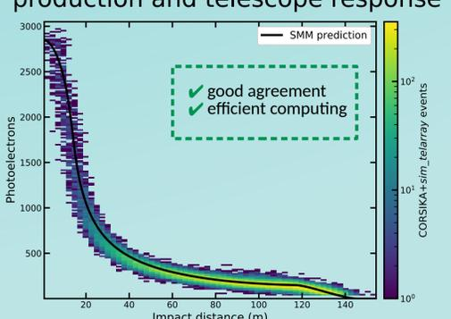
Figure 1: Number of photoelectrons collected by the telescope camera as a function of impact distance. The prediction of the SMM is compared to that of a full simulation [2]
