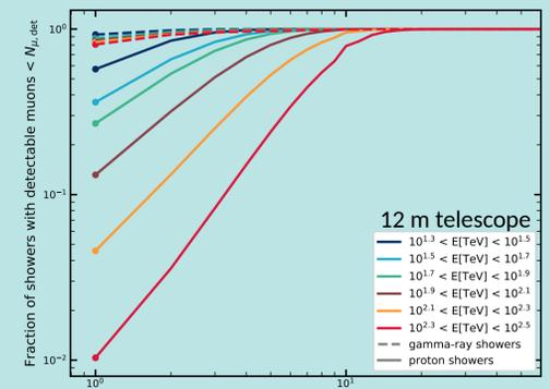
Figure 3: Analogous to Fig.2 for a 12 m telescope. The rejection capability is much worse due to the reduced light-collection area.
