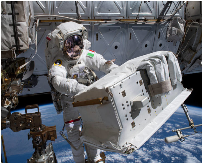
Luca Parmitano during the installation of the AMS-02 UTTPS.
