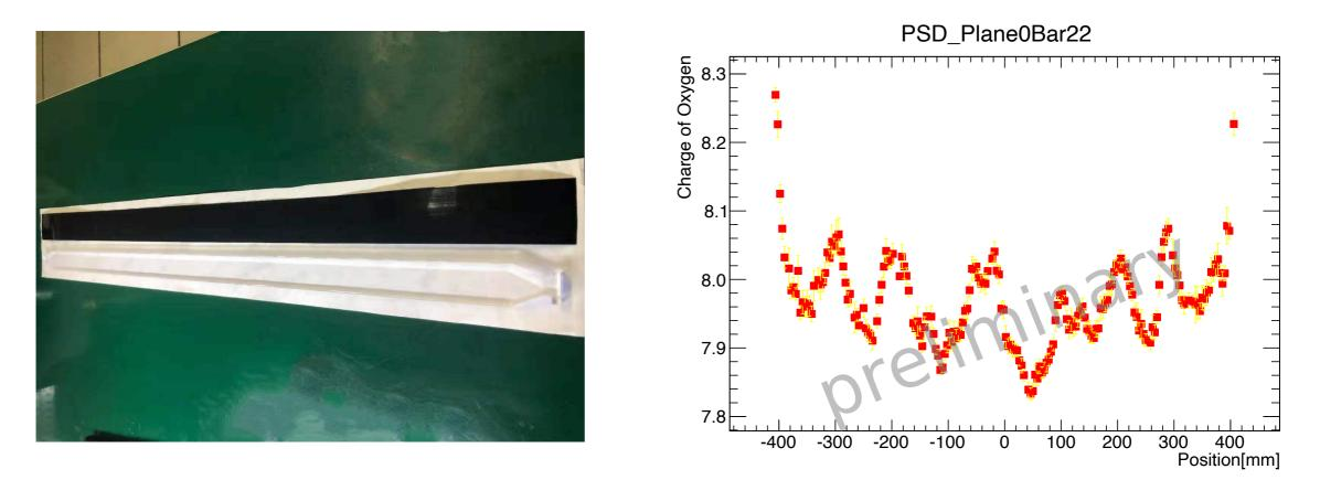
• This feature is due to that light reflection material Tyvek paper did not attach to the surface of scintillator bar uniformly
