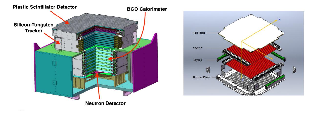
• PSD is composed of two orthogonal planes, with 41 units in each plane.
