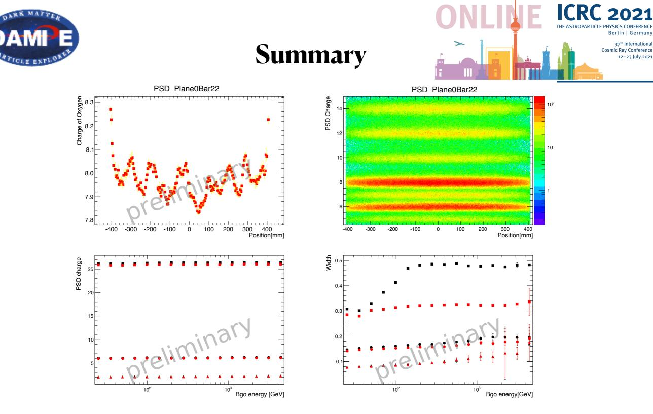
• We eliminate PSD charge variation versus hit position, the correction is helpful to measure the spectra of GCR heavy components.
