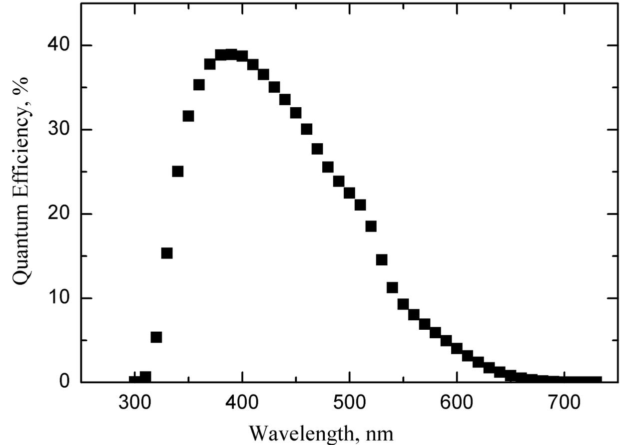
Quantum efficiency reaches almost **40%** at **390 nm**
