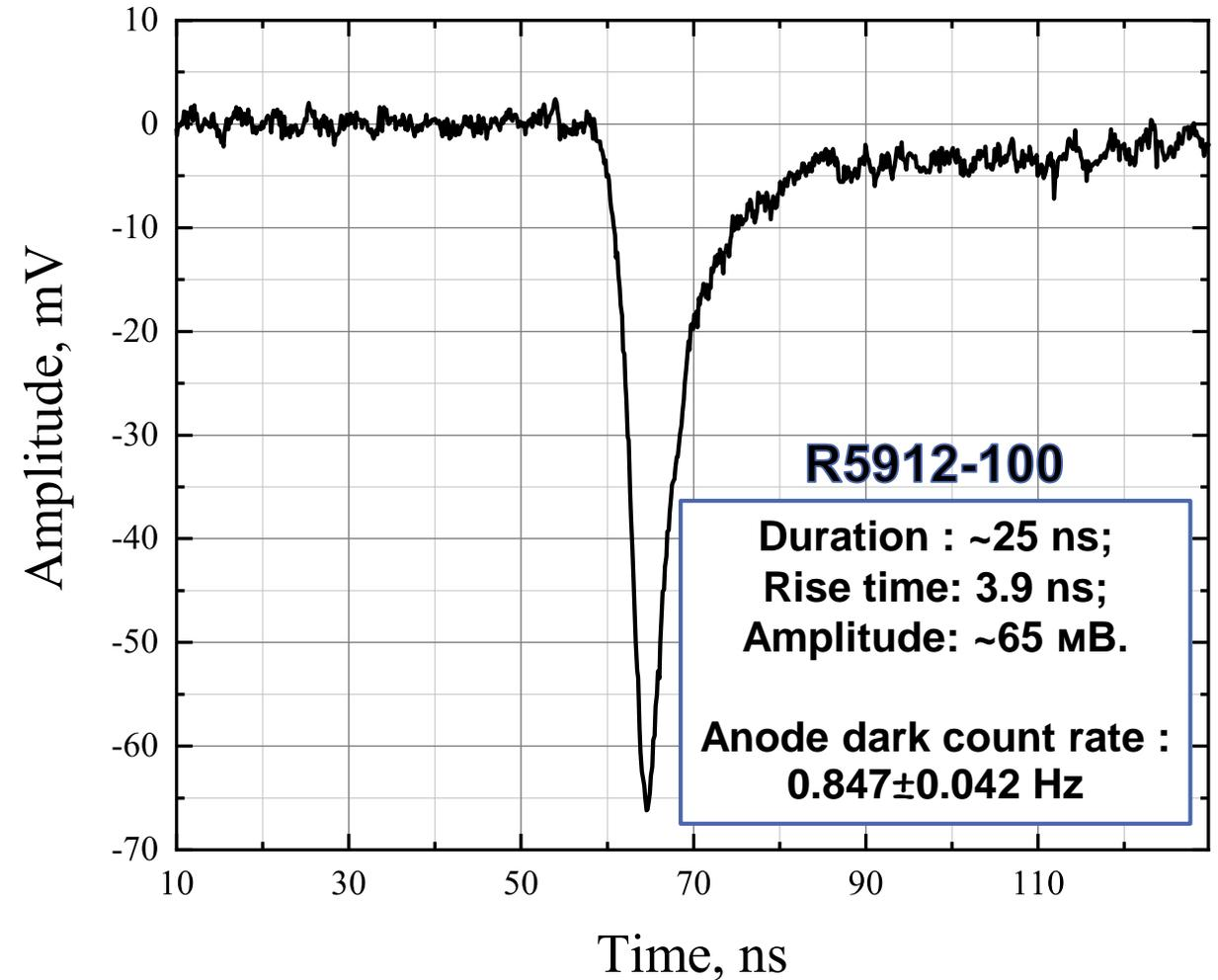
The SPE pulse waveforms with a PMT gain of  $\sim 10^7$  and an amplifier gain of 10.
