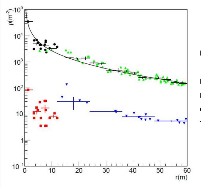
Lateral distribution of the coincident event. Red square: neutrons by ENDA. Blue triangle: muons By KM2A-MD. Black dot: electrons by ENDA. Green triangle: electrons by KM2A-ED. The black line is NKG function fitting.
