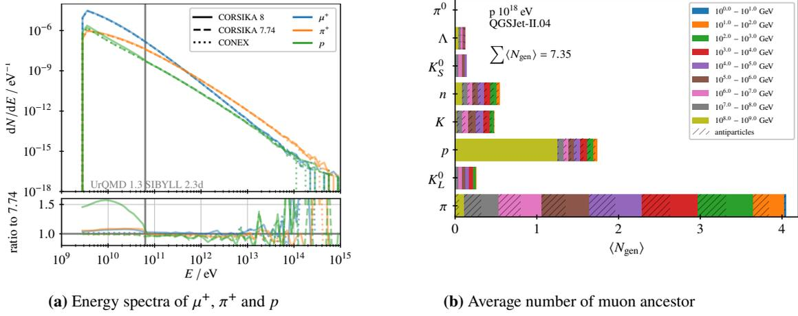
**Figure 2:** On the left, the energy spectra of  $\mu^+$ ,  $\pi^+$  and  $p$  of  $1 \times 10^{17}$  eV vertical proton shower, averaged over 400 events. On the right, the average number of muon ancestor projectile generations by particle species and energy.
