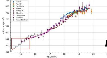
Mean depth of maximum of EASs vs. energy of primary cosmic rays according to data of different experiments. The black triangle shows estimations for the TUS161003 event.
